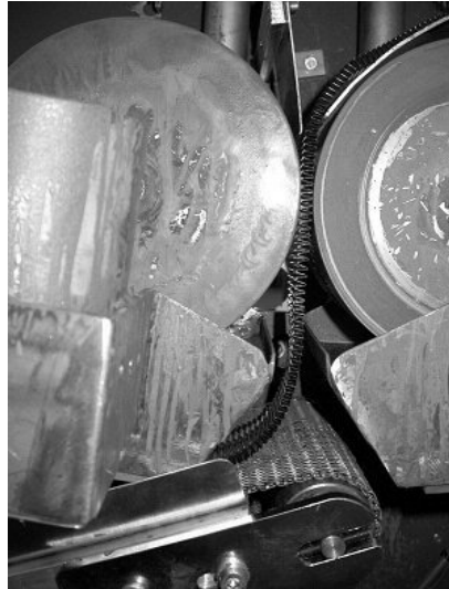
Figure 16. Fin-tip coating in practice.
