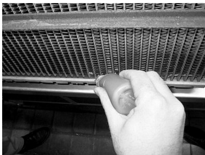
Figure 18. Manual applying of header paste.
