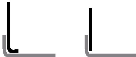
Figure 29. Alternative joint geometries for header-tank.
