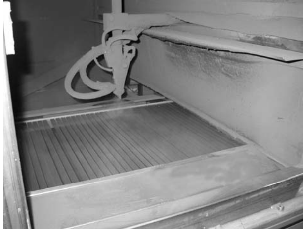
Figure 14. Automatic spraying of paste on radiator tubes. Both sides are sprayed simultaneously. The picture shows the upper spray gun.
